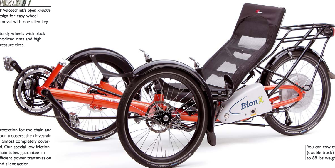
Due to the low centre of gravity and the well balanced weight distribution the Scorpion handles fine even when braking hard. The standard disc brakes offer great stopping power, allowing for a fast yet safely controllable downhill ride. Each wheel has its own brake lever so you can concentrate the braking power at the inner wheel in sharp turns. HP Velotechnik's famous steering geometry avoids any unsafe brake steer or bump steer. Optional coupled front brakes for one-hand operation of both brakes.
